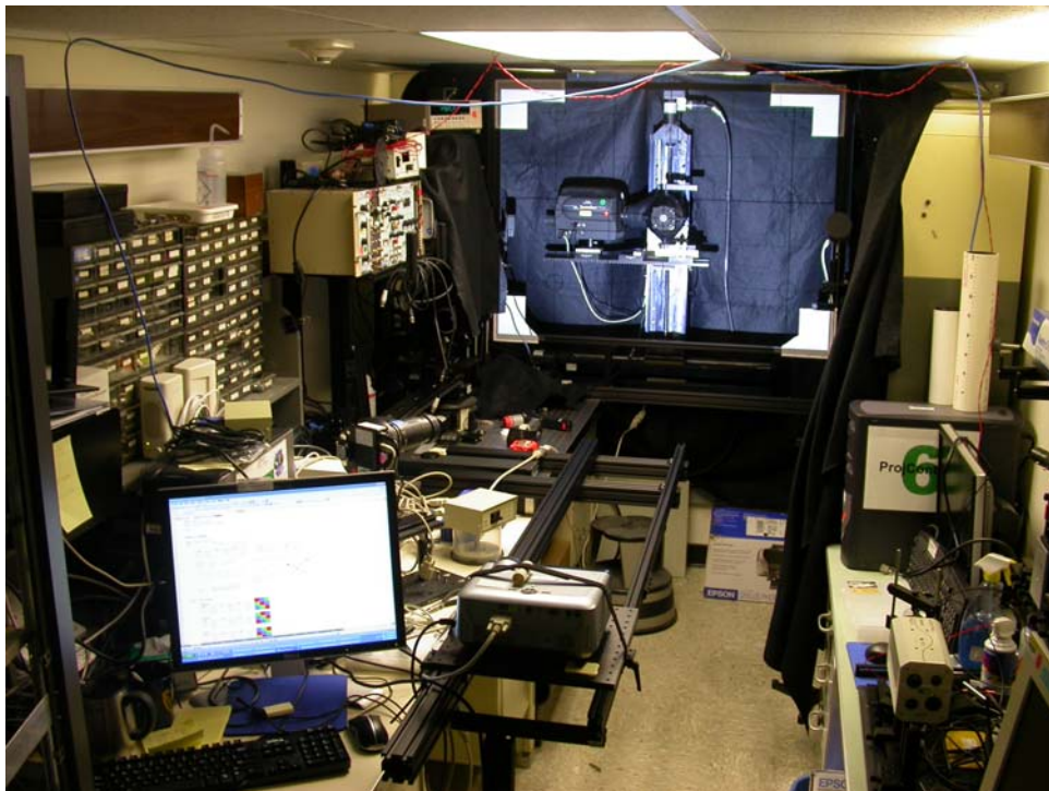
Figure 6. Laboratory setup. The projectors are placed on a rail system for positioning. The video generator is outside of the picture at the left.
