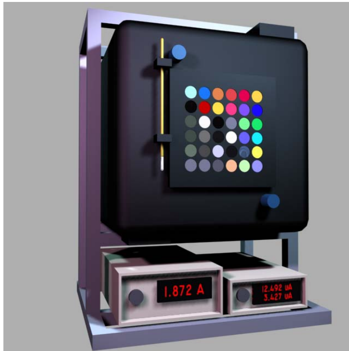
Fig. 1. Each DMATS unit will consist of a uniform illumination source with a suite of optical targets mounted in a removable, reconfigurable faceplate. The unit will be shipped with power supply, photodiode monitors and picoammeters, digital thermometer, and a laptop computer for automatic logging of photodiode current and operating temperature.
